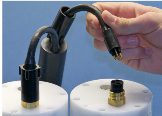
Figure 2. Beware of a short-circuit hazard in this situation: when one branch of the Y-cable is connected to a HydroBatt, the male pins of the other branch carry the first battery's output voltage!
