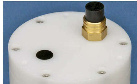
Figure 3. The black circle on the left of the end cap is the top of the pressure relief valve. Never block the valve. If it pops up, that indicates a possible hazard and you should discontinue use.
